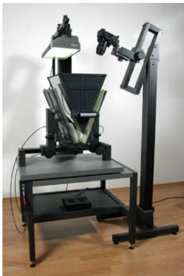
Figure 1. Book cradle for 45 degrees photos (Source: www.image-engineering.de ).
